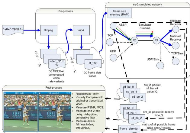
Figure 1. Overview of the simulation environment (pre-processing, ns-2, post-processing)
