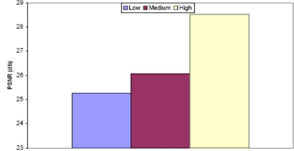
Figure 20. PSNR values of the received MPEG-4 video (Average PSNR: Low=25.26 dB, Medium=26.06 dB, High=28.52 dB)
