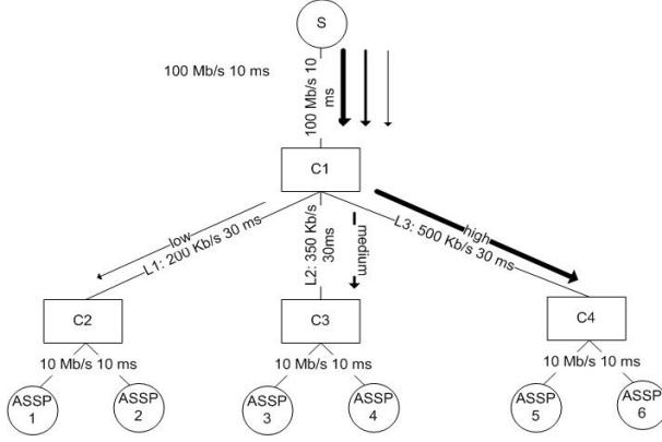
Figure 2. Topology for stream accuracy subscription
