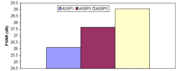
Figure 7. PSNR values of the received MPEG-4 video (Average PSNR: ASSP1=26.11 dB, ASSP3=27.64 dB, ASSP5=29.05 dB)
