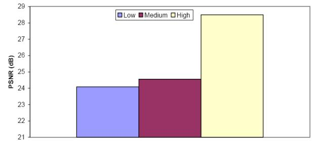
Figure 12. PSNR values of the received MPEG-4 video (Average PSNR: Low=24.09dB, Medium=24.56 dB, High=28.05 dB)
