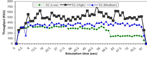
Figure 14. Achieved throughput of ASSP receivers that join the second ASSP source
