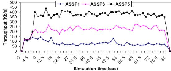
Figure 3. Achieved throughput of the three multicast receivers (ASSP1: low connection (83 Kb/s), ASSP3: medium (221 Kb/s), ASSP5: high (360 Kb/s)
