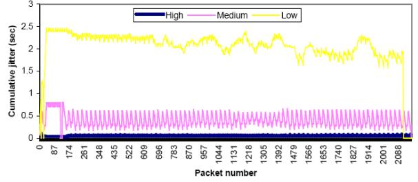
Figure 19. Cumulative jitter of the three ASSP flows
