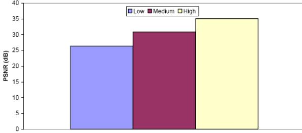
Figure 16. PSNR values of the received MPEG-4 video (Average PSNR: Low=26.36 dB, Medium=30.83 dB, High=35.06 dB)
