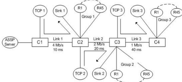
Figure 8. Network topology for TCP-fairness simulation
