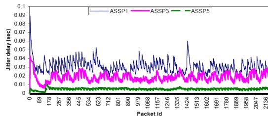
Figure 5. Delay jitter of the three ASSP flows
