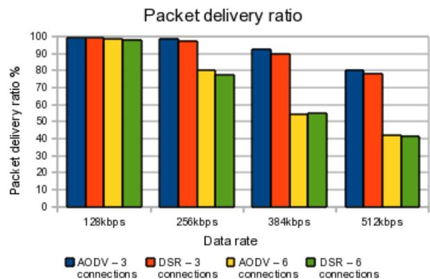
Figure 5. Delivery ratio over different data rates
