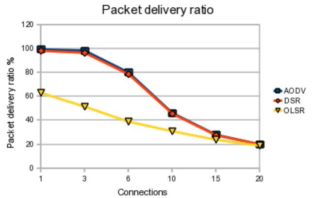
Figure 1. Delivery ratio over different maximum connections
