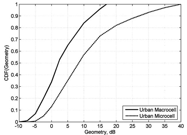
Fig. 2 Geometry CDF macrocell-microcell
