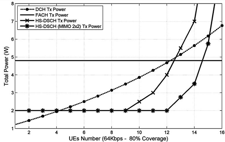
**Fig. 7** MBMS power allocation, 64 kbps, 100% coverage
