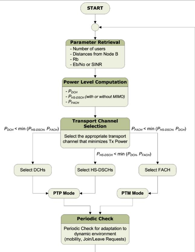
Fig. 4 Power counting mechanism with MIMO functionality
