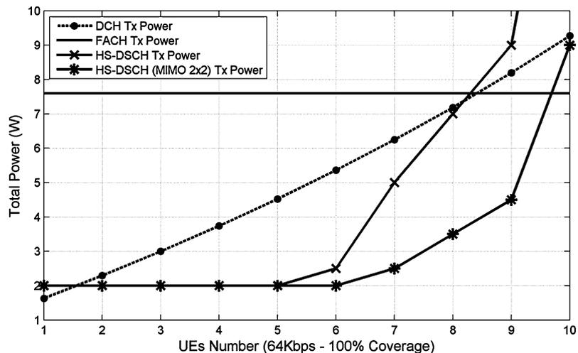
In general, in cases where the number of users is small, PTP transmissions are preferred. DCH and HS-DSCH are both PTP channels; however, the results prove that for very small multicast user population DCH is preferred, while, for relatively more users HS-DSCH is the most appropriate. Therefore, our mechanism does not only decide to use PTP or PTM transmissions (as the existing Counting Mechanism does), but it makes a further distinction between DCH and HS-DSCH in PTP mode.
