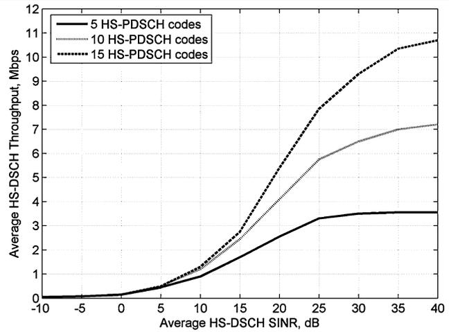
Fig. 1 Actual cell throughput vs. *SINR*
