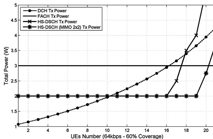
**Fig. 6** MBMS power allocation, 64 kbps, 80% coverage
