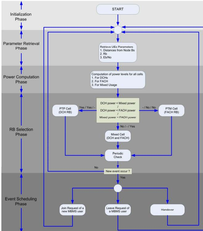
Fig. 1. Block diagram of the proposed power control mechanism
