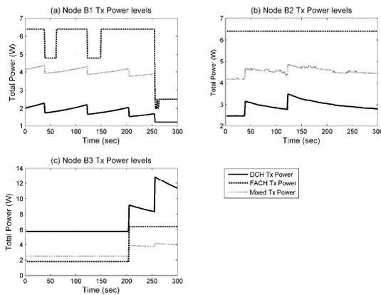
Fig. 4. Transmission power levels of cells under study during handover
