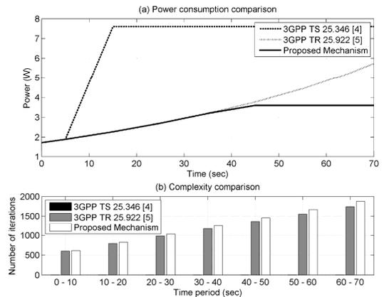
Fig. 5. (a) Power consumption and (b) complexity comparison
