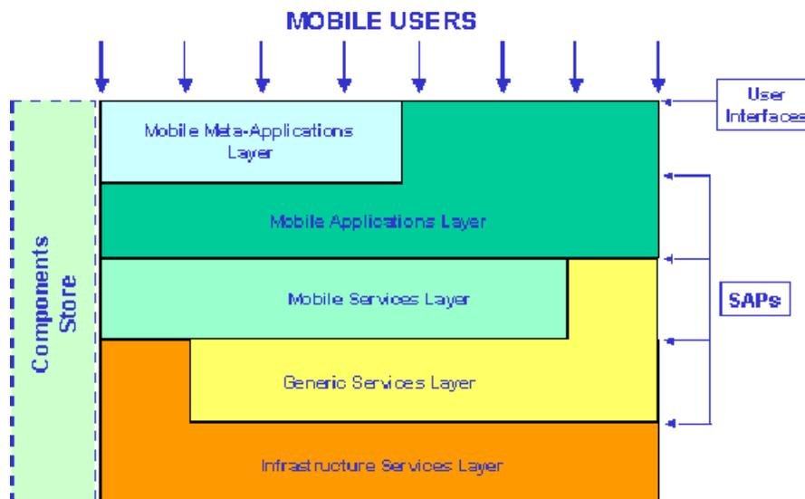
Figure 3. The OMAF layered-model
