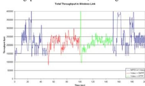
Figure 9. Total throughput in Wireless Link (with background traffic)
