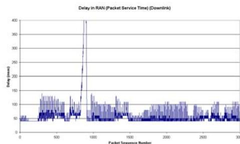
Figure 5. RAN delay for the Video Transmission
